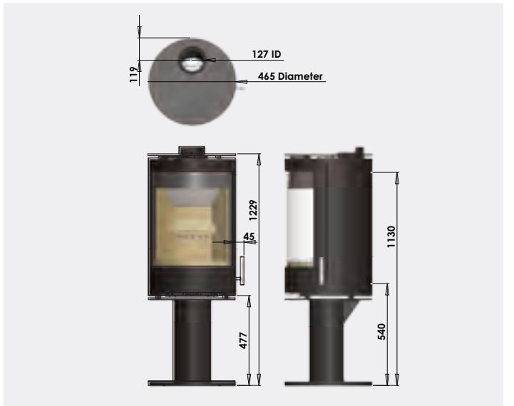
BPVR cylinder on high pedestal stand
