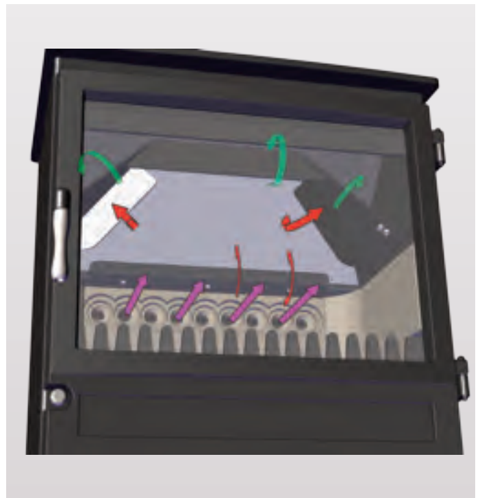
Purevision Heritage Airflow Diagram
